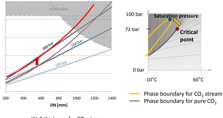
Wall thickness for CO<sub>2</sub> stream
