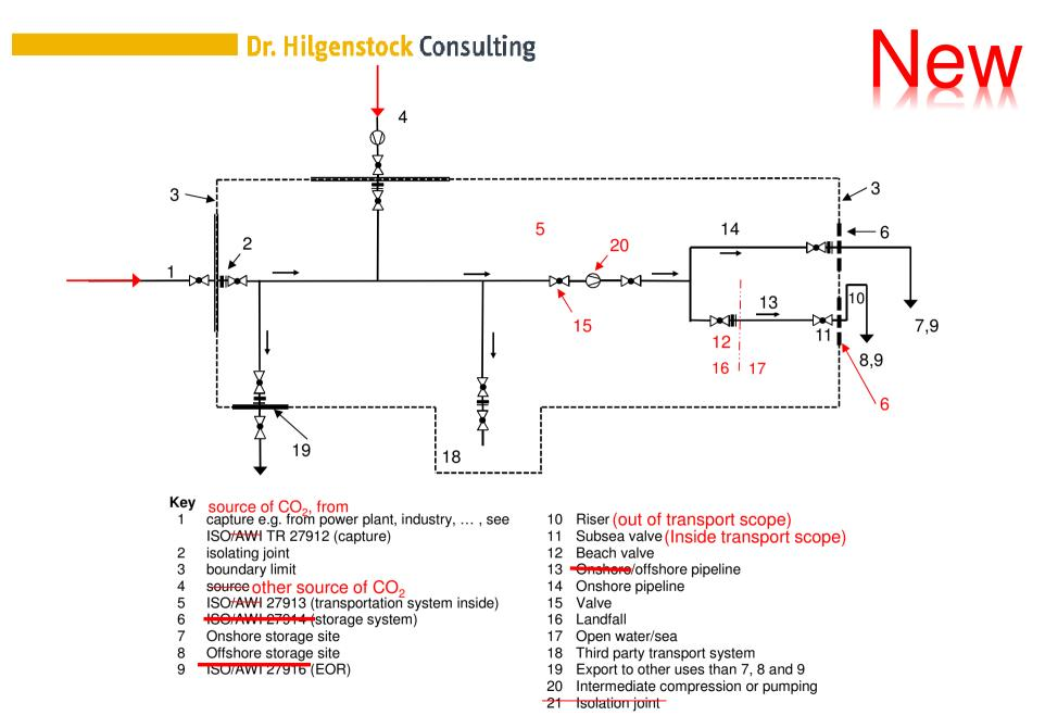
Figure 1 — Schematic illustration of the system boundaries of ISO 27913
