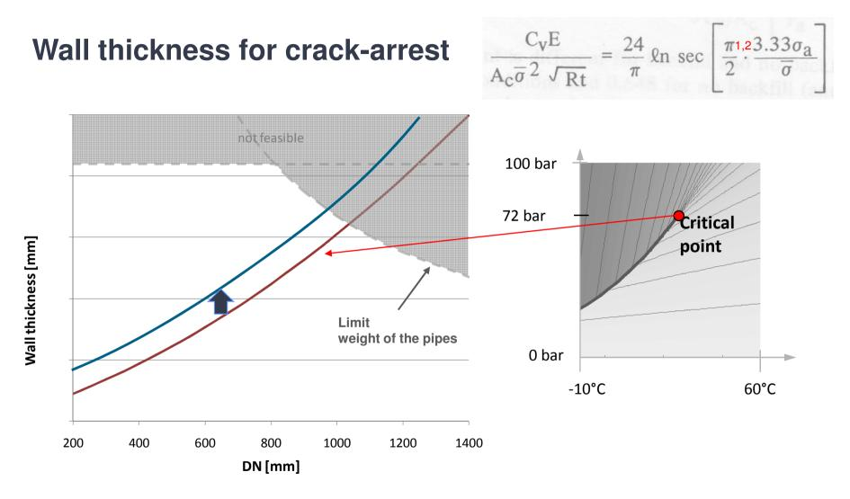
Parameters: Steel X 70, Cv > 100 J Driving pressure at critical point
